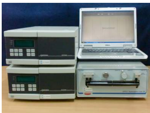
Fig. 1 On-line Personal OSU50 Isocratic OPLC Chromatograph with ECOM ECP2010 Pump, ECD 2600 UV-VIS Detector and DataApex Clarity Chromatography Software
